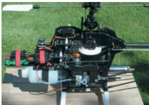
Right side and rear bellcranks seen here, all are double ball raced.
