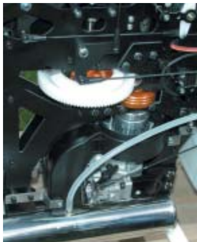
Right side and rear bellcranks seen here, all are double ball raced.
